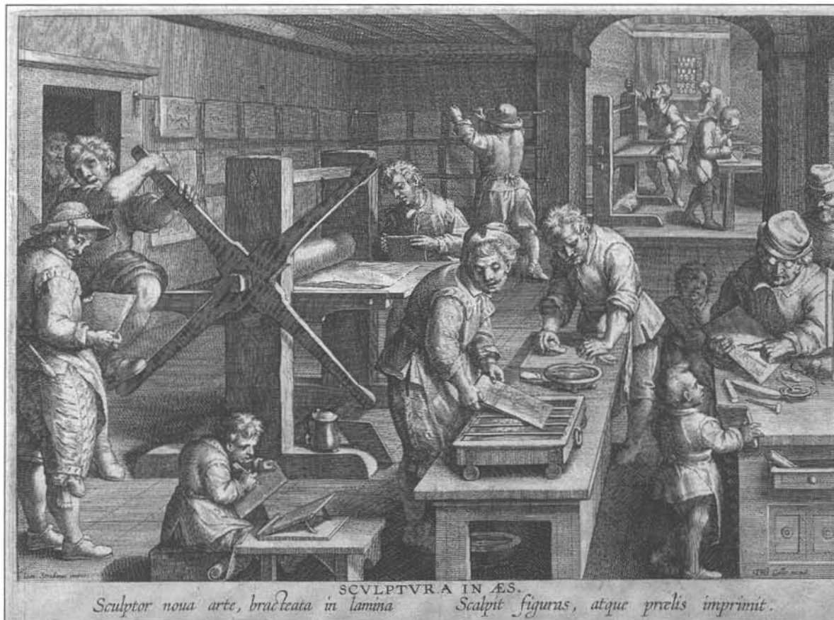
Figure 2. An early copperplate printing shop illustrated in a copperplate print by Stradanus (1590). Copperplate prints, including maps, were printed using a large rolling press as shown in this illustration. From an original in the author's collection.
